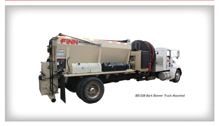
FINN Bark Blowers apply landscape mulch and other bulk materials with unprecedented efficiency, and eliminate the need for labor-intensive hand application. The BB1208, with 8.2 cubic yard capacity, the BB1216, with 15.7 cubic yard capacity and the BB1222, with 21.8 cubic yard capacity, provide high efficiency mulch application capabilities for landscape maintenance companies and mulch suppliers.
