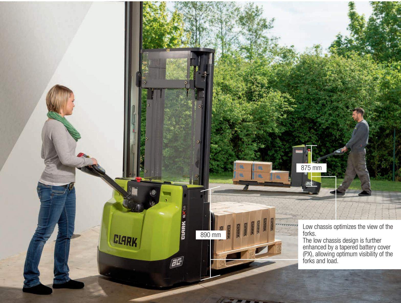
Low chassis optimizes the view of the forks. The low chassis design is further enhanced by a tapered battery cover (PX), allowing optimum visibility of the forks and load.
