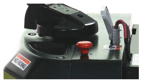
**Packed with safety features.** The WSRX features an emergency stop button within easy reach of the operator, electronic brake when the handle is raised and speed control when the forks are raised above 30cm. Neutral resisting roll back on ramps, safety reversing belly button to prevent crush injury and easy access horn are additional features that make the WSRX safe whilst remaining versatile.
